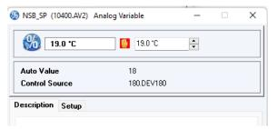
The night setbacks for other units are calculated using various equations. In some cases, the logic refers to undefined values which may result in unpredictable results.
