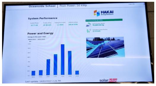
Figure 4: Solar PV Dashboard
