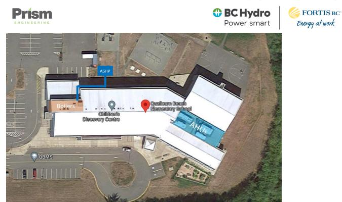
Figure 22: Possible alternative locations for an air-source heat pump connected to the heating loop
